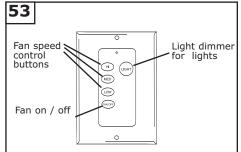
To control fan speed select from high, medium or low speed buttons. To turn the fan off press the Fan on / off button. To dim lights press and hold light button. To turn off light press and quickly release button.
